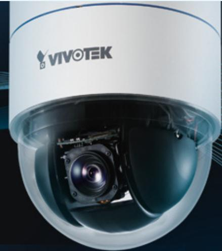
VIVOTEK SD8111/21, equipped with a 12x optical zoom lens, is a high performance day/night speed dome network camera geared for professional surveillance applications, representing another significant addition to VIVOTEK's high-end H.264 network camera portfolio.
