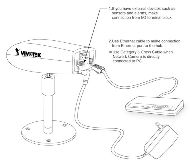
3. Finally, connect power cord to a power outlet
