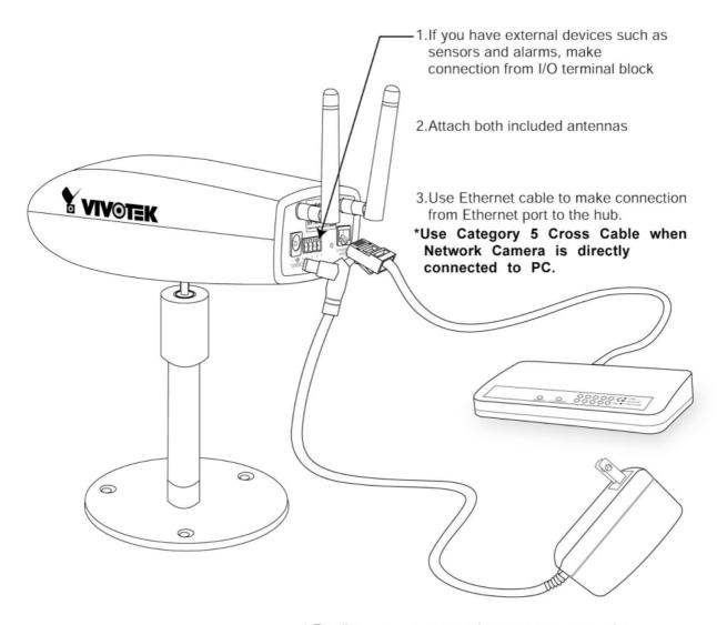
4. Finally, connect power adapter to a power outlet
