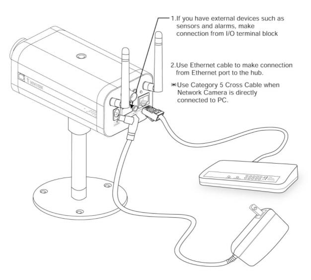
3. Finally, connect power cord to a power outlet
