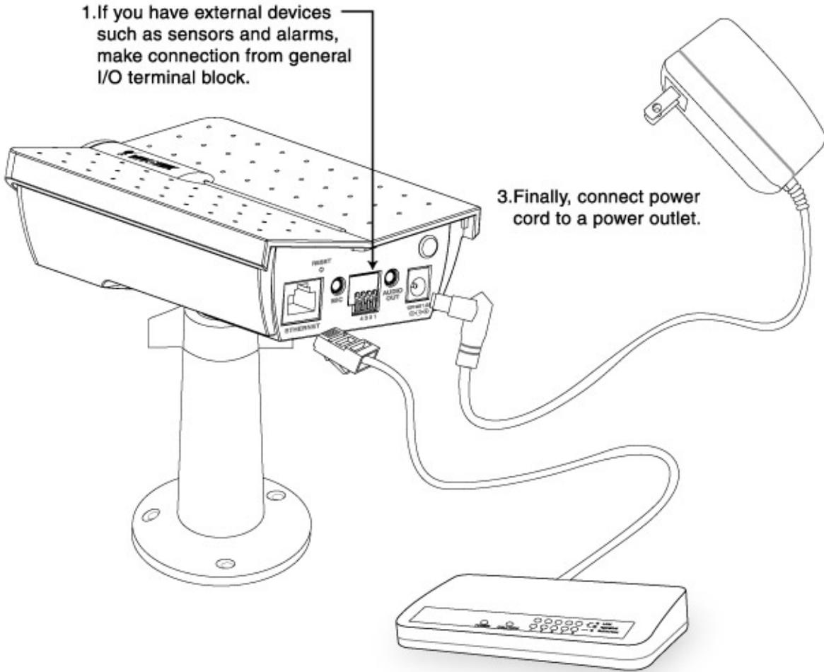
1. If you have external devices such as sensors and alarms, make connection from general I/O terminal block.
