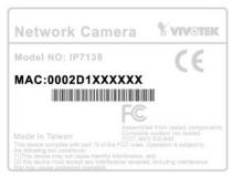
This serial number is same as Ethernet address, for example: 0002D1100052=00-02-D1-00-00-12
