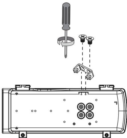
**16.** Install the housing to the wall-mount bracket by aiming and pressing the spring mortise, and hook the bracket onto the groove in the spring mortise.
