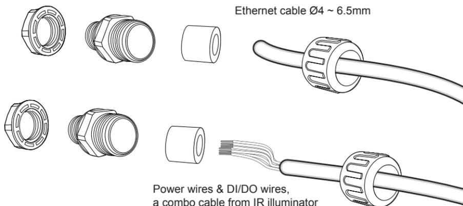
You may need to remove the RJ45 connector, and use a crimping tool to connect the Ethernet wires to an RJ45 connector inside the enclosure. Use an Ethernet cable of the width of 4 ~ 6.5mm.
