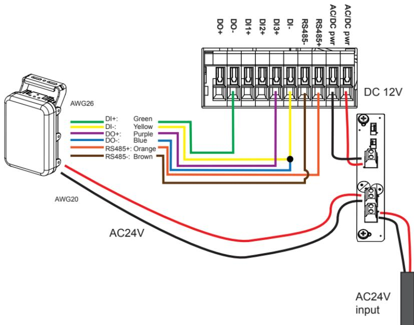
**14.** You can connect the ground wires together and connect them to the DI- ground pin on the terminal. Use a small flat blade screwdriver to press the lever on the terminal block.
