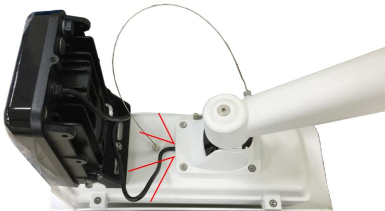
**17.** Secure the housing to the bracket by fastening 4 T30 screws.
