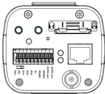
The day/night mode DI connection enables the synchronization of IR light and the automated day/night switching mechanism on the camera.
