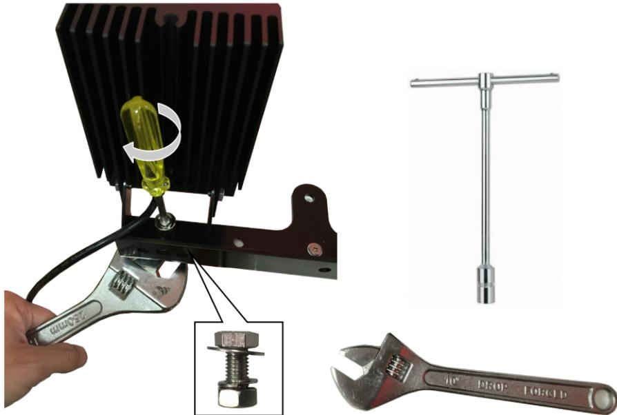
Secure both IR light units to the included iron bracket in the orientation shown below.
