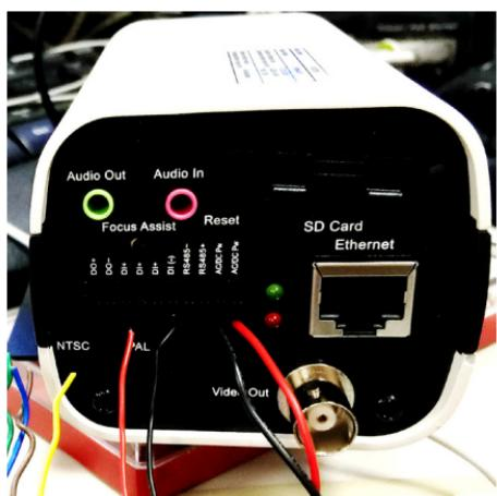
The day/night mode DO connection enables the synchronization of IR light and the automated day/night switching mechanism on the camera.
