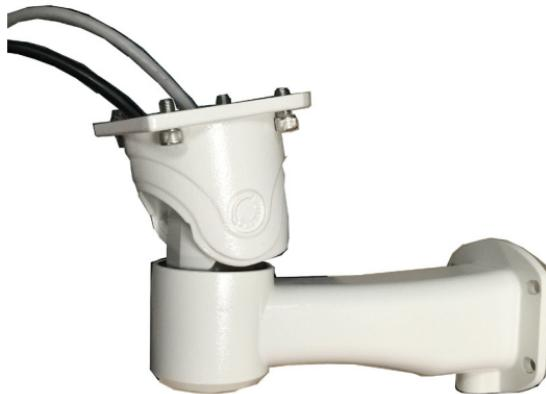
**17.** Mount the enclosure on to the installed bracket, and secure the connection by tightening the 4 socket screws. Due to the weight of the enclosure (5.5kg), it is best to have two men mounting the enclosure.
