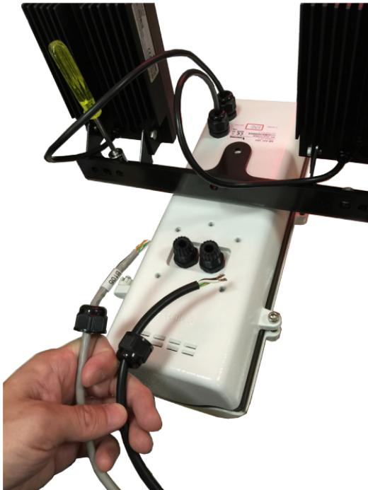
You may need to remove the RJ45 connector, and use a crimping tool to connect the Ethernet wires to an RJ45 connector inside the enclosure. Use an Ethernet cable of the width of 5 ~ 6.5mm.
