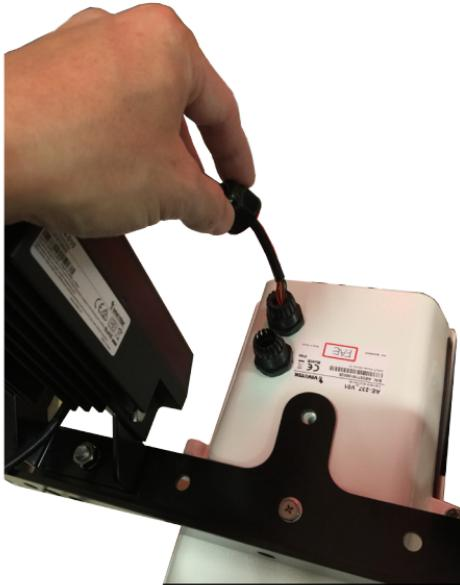
6. Loosen the retention hex screws of the enclosure. To access the screws, you can push the IR bracket to the side.
