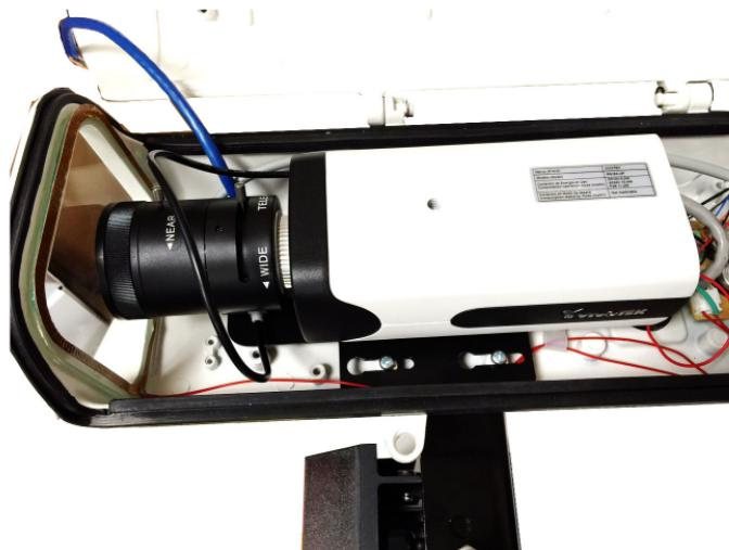
**19.** Close the top cover of the enclosure, tighten the screws, and secure another screw to the IR bracket.
