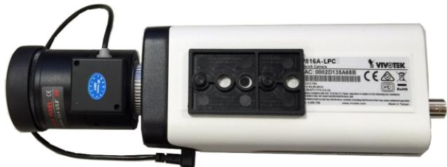
**11.** Place the mounting plate on top of the buffer pad and then secure it to the camera. You may need adjust its position so that the lens module can flush align with the tempered glass.
