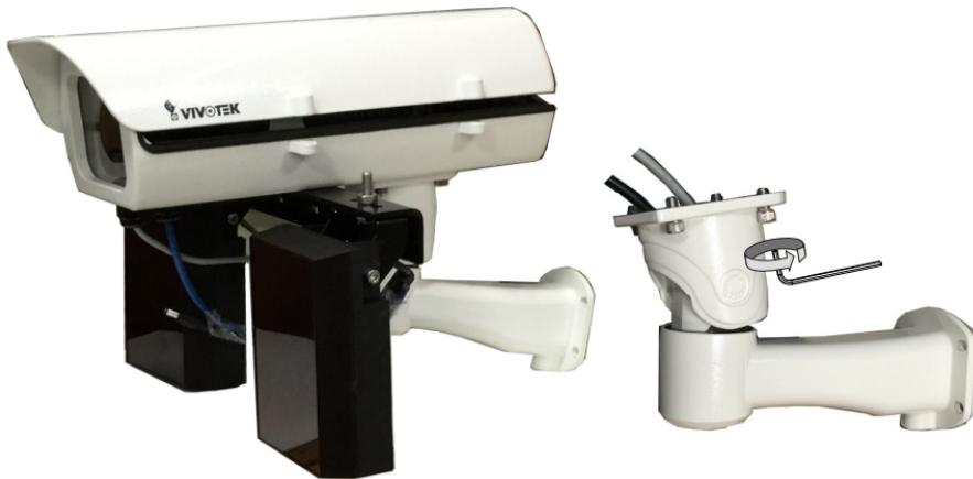
**18.** Adjust zoom and focus and open a web session with the camera to tune for the best image. When zoom and focus is done, Close the top cover and fasten the top cover screws.
