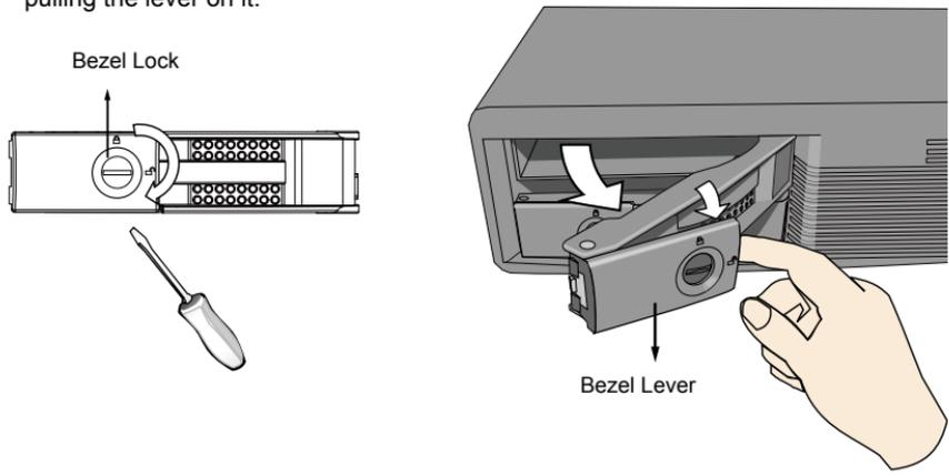
2. Install your hard disk to the drive bay. Gently put the hard disk into drive bay with its label side facing up and the connector side towards the inside of the chassis. Push the hard disk in. Stop pushing it when you feel the contact resistance.
