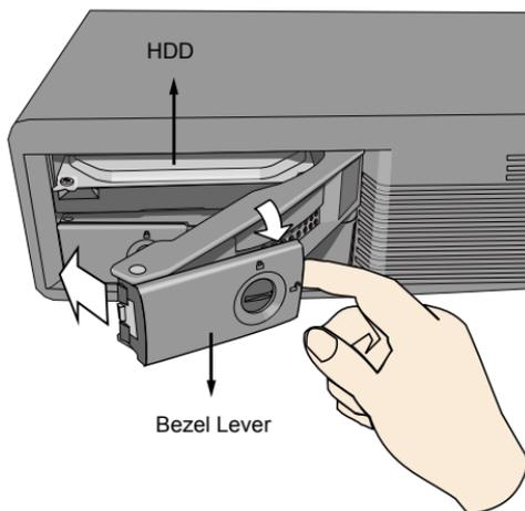
4. 4-1. Press on the left edge of the drive bay bezel to snap it into place.
