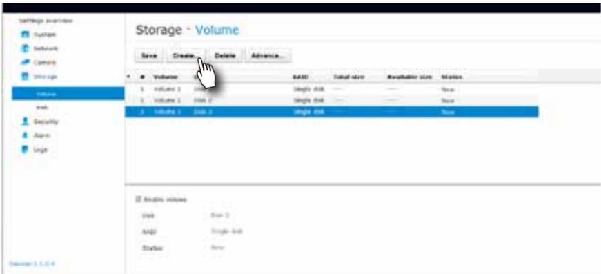
9. Depending on the number of hard drives you installed, a list of RAID volume configurations will be listed. Select a configuration's check circle and the disk members of a volume, and then click **OK** to continue. The initialization of a RAID volume will take several minutes.
