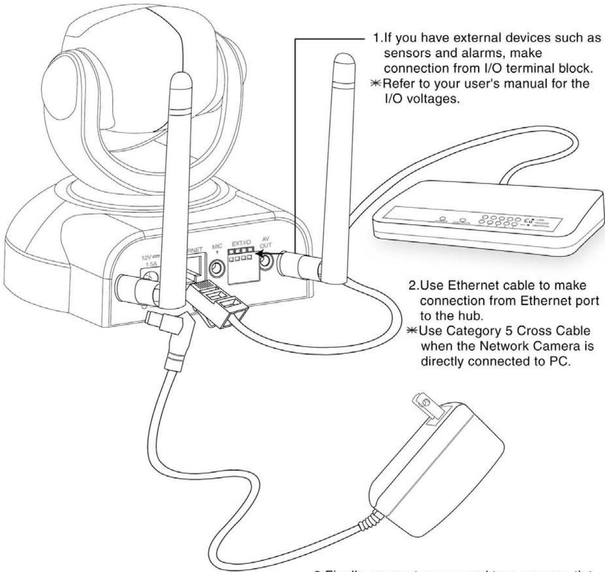
1.If you have external devices such as sensors and alarms, make connection from I/O terminal block.
