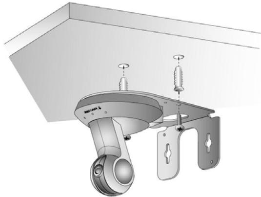
3. If adopting POE kit (optional accessory), the POE splitter can be attached to the bracket by using the two supplied screws (typeB).
