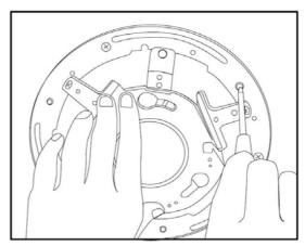
6.Connect the data cable and Ethernet through the center hole of the Mount to the dome body.
