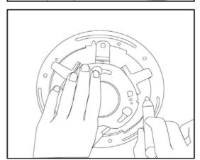
5. Fix the Mount with three screws.
