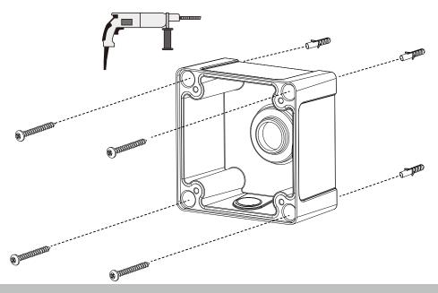
4. If you need to route cables through a conduit, remove the plastic stopper underneath the junction box.
