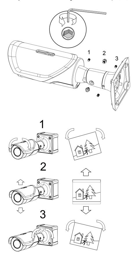
15. Tighten the retention screws when you are statisfied with the field of view.
