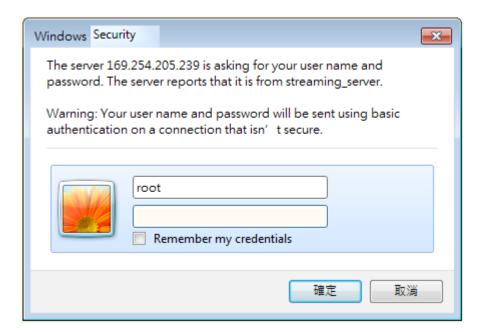
13-2. Enter the combination of alphabetic and numeric characters to fulfill the password strength. requirement. The default name for the camera administrator is "root", and can not be changed.
