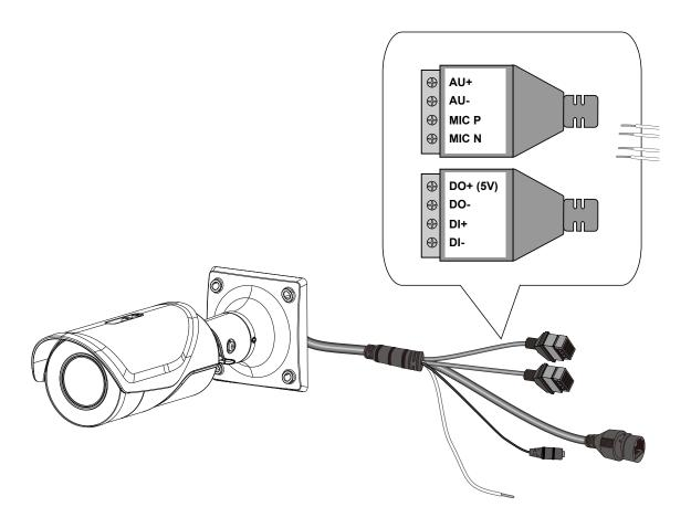
8. Pass an Ethernet cable through the waterproof cable gland components, and through the rubber seal as shown below. Connect the Ethernet cable to the camera's RJ45 onnector.
