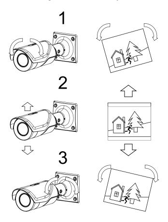
16. Tighten the retention screws when you are statisfied with the field of view.
