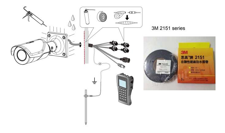
It is also very important to route cables to form a drip loop. Leakage or moisture can gather in condensation into water drops and run along the cable. A drip loop ensures no water gets to the camera.
