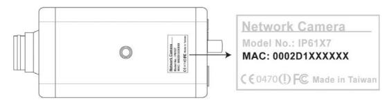
This serial number is the same as Ethernet address, for example: 0002D1140000=00-02-D1-14-00-00
