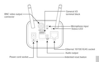
Please verify that your product package contains all the accessories listed in the foregoing Package Contents. Depending on the user's application, an Ethernet cable may be needed. The Ethernet cable should meet the specs of UTP Category 5 and not exceed 100 meters in length.
