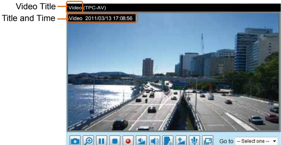
**Video orientation:** Flip--vertically reflect the display of the live video; Mirror--horizontally reflect the display of the live video. Select both options if the Network Camera is installed upside-down (e.g., on the ceiling) to correct the image orientation. Please note that the e-PTZ preset locations will be cleared after flip/mirror.
