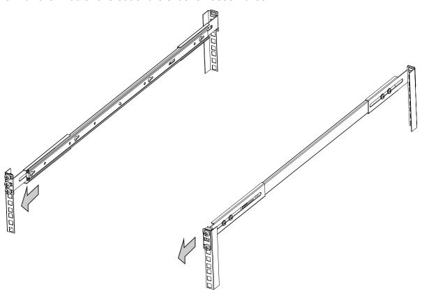
7. Hold the chassis using both hands on the sides of the chassis. Align the tips of inner rails on the chassis with the open portion of the slide rail assemblies. Push the system into the assemblies until the system stops.
