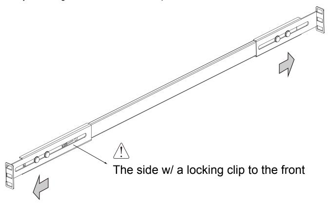
5. Secure the slide rails to rack posts using the #10 screws.
