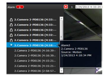
The alarm panel is polled every 10 seconds. A mouse hover on an alarm entry displays full information of the event
