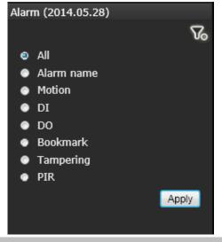
If you set up multiple triggering sources on a camera, you can use the **Alarm filter** button to find the alarms of a specific type.
