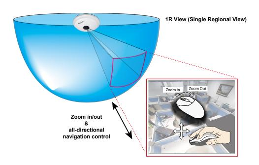
The 1R mode (or rectilinear) provides access to one image section within the hemisphere. You can zoom in or out (using the mouse wheel or PTZ panel) or travel through to other areas within the hemisphere using simple mouse clicks and drags. A single click on a particular object can bring the object to the center of your view window. Click and hold down the left mouse button, and you can swipe the view both horizontally and vertically.
