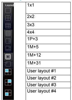
By default, 5 typical layouts are provided for the user. They include: 1x1, 2x2, 3x3, 4x4, 1P+3, 1M+5, 1M+12, and 1M+31. System default is the 4x4 layout. Cameras that do not fit into the first page of a layout, say, a 3x3 layout, will be displayed on the succeeding layout pages.
