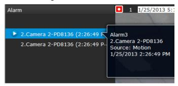
The alarm playback window will begin playback of a footage taken **10 seconds** before the occurrence of an alarm. The playback of an alarm-triggered recording will normally last for **one minute**. If, however, you configured a shorter pre- and post-alarm recording time, your alarm recording may be slightly shorter. The default for **pre-** and **post-alarm** buffer time are 5 seconds and 20 seconds.
