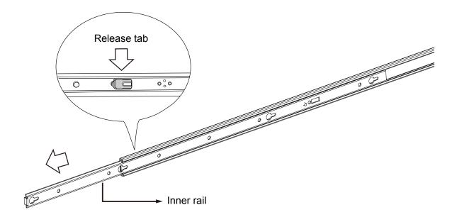
3. Secure the inner rails to the sides of the chassis using the M4 screws.
