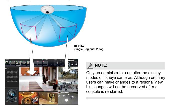
In addition to fisheye cameras, if a camera has a wide field of view, you may also display its different fields of view in multiple view cells. Some view cells may also contain a PiP view that is digitally zoomed.
