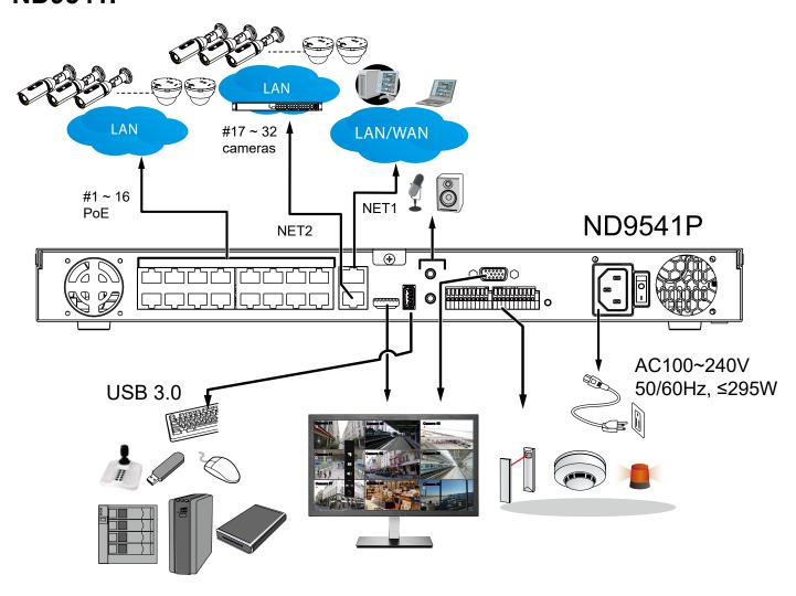
ND9541P supports 32 channel recording, and the onboard 16 PoE ports supply power and data connectivity for 16 cameras. The NET2 GbE port should be used to connect another 16 cameras in a local network via a PoE switch or mid span.
