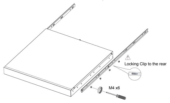
4. Secure the L-shape brackets to the front- and rear-ends of outer rails using the **black** round head screws and washers. Do not completely tighten the screws yet. Adjust the length of slide rails by extending and matching the rails between rack posts.
