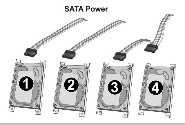
5. Secure the hard disks to the mounting positions in the chassis with its label side facing up, and the connectors facing the inside of the chassis. The sample drawing below shows the position of drive #2.
