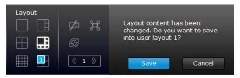
5. You can create more user layouts by mouse-overing the user layout button. You may create more user layouts for different purposes, such as for the use of different users, or playing different views of a camera on multiple view cells.
