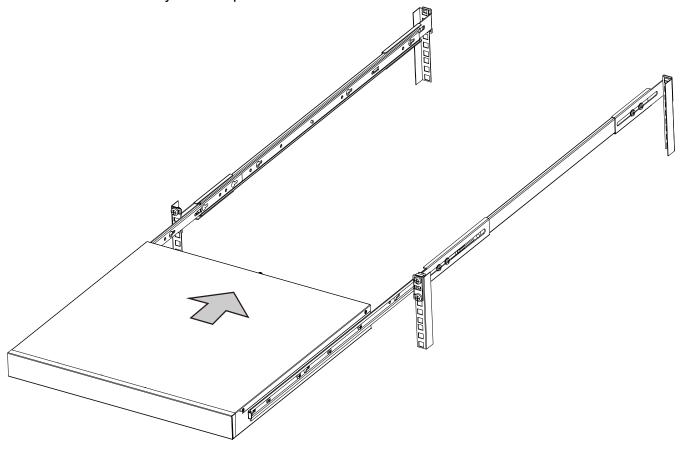
8. The inner rails and the rail assemblies should be locked on the way into the rack cabinet. Press the release tabs on the sides to slide the chassis into rack.
