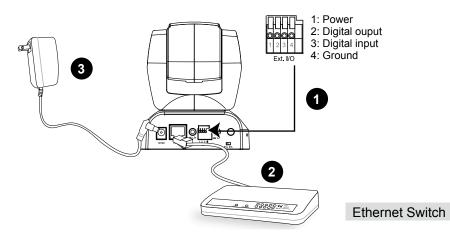
There are several ways to set up the Network Camera over the Internet. The first way is to set up the Network Camera behind a router. The second way is to utilize a static IP. The third way is to use PPPoE.
