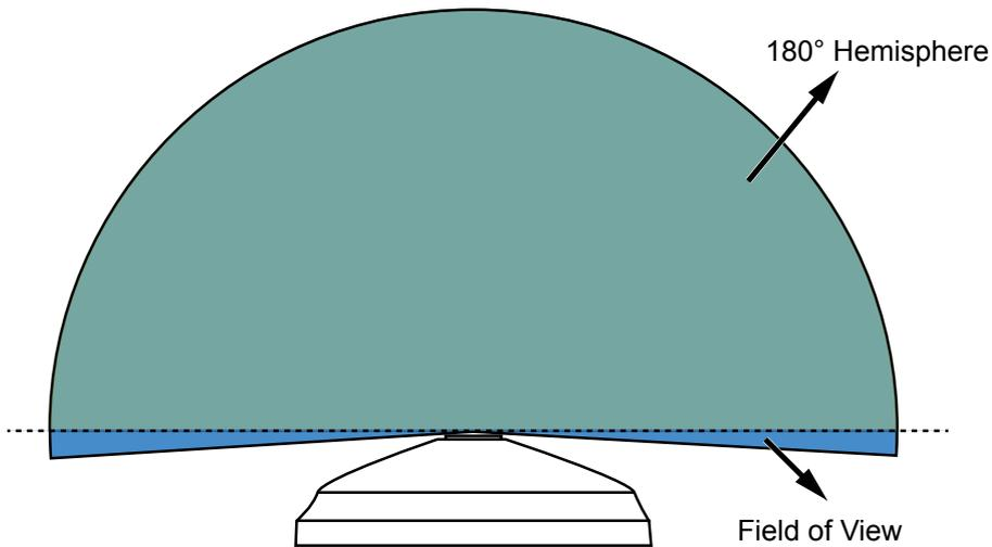
1. Edges of a fisheye circular view will be slightly cropped because the fisheye lens FOV is larger than the sensor can take.
