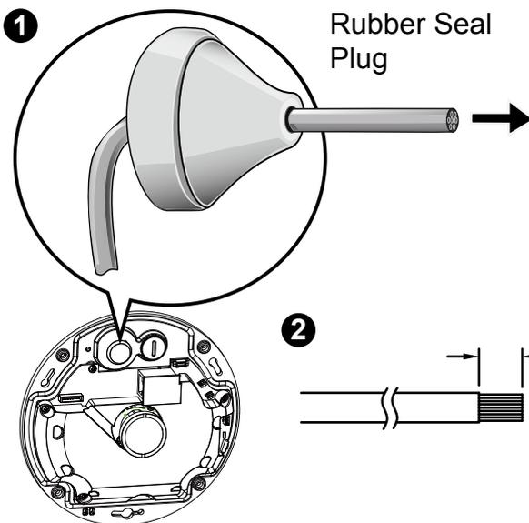
1. Drill a hole on the rubber seal plug and insert an Ethernet cable through the opening.
