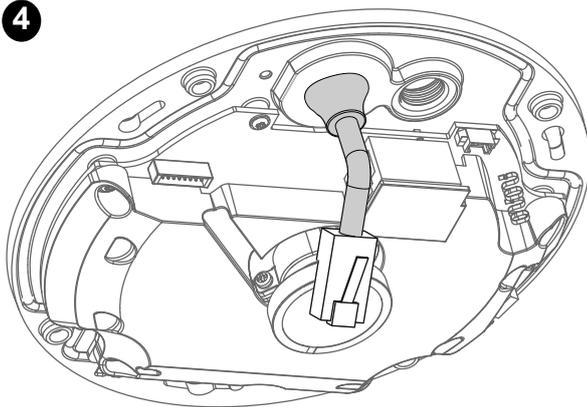
4. Feed the Ethernet cable from the bottom of the camera and through the hole. Attach the rubber seal plug for water proofing.
