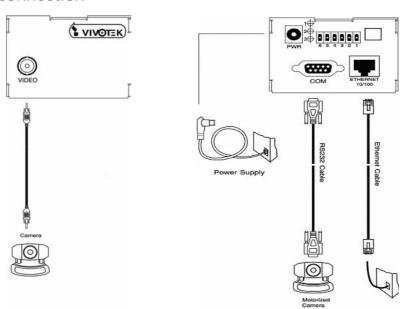
Shut down all the peripheral devices prior to connection. The video BNC, Ethernet cable and power adapter are essential for basic viewing function. If the attached cameras belong to the same motorized model, they can be concatenated to single COM port and will be differed by camera ID set on the cameras. Refer to the related configuration section for detailed description.
