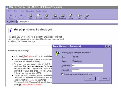
Through direct connection by null modem cable, administrators can connect to "http://200.1.1.1" in the web browser. "200.1.1.1" will be the default IP address of Video Server in dial-in connection; "200.1.1.100" will be the given IP address for the user's PC by Video Server. The user name and password are the same as what was entered during software installation.
