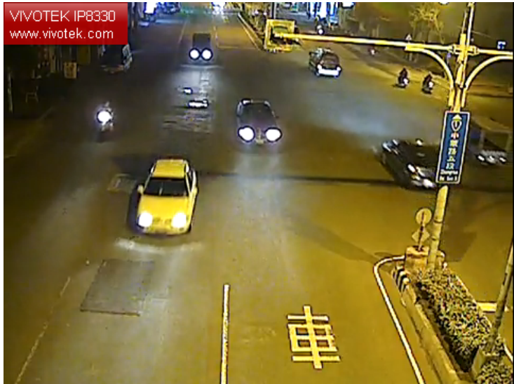
Fig. 2 A low lux rated camera can capture clearer nighttime video, even without any additional external lighting.
