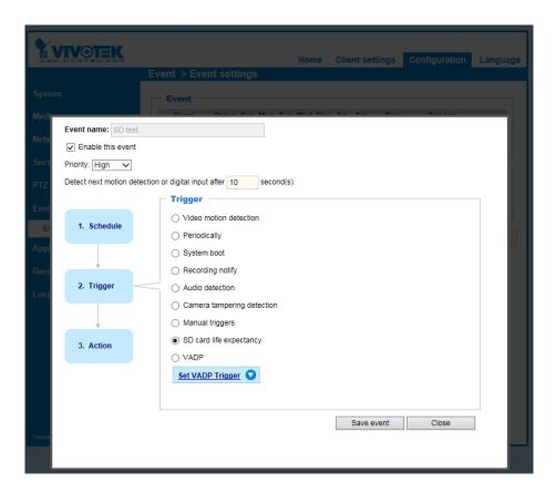
In the Event settings > Action page, create a media type as the "System log." The system log will be delivered to users when an SD card related event is detected.
