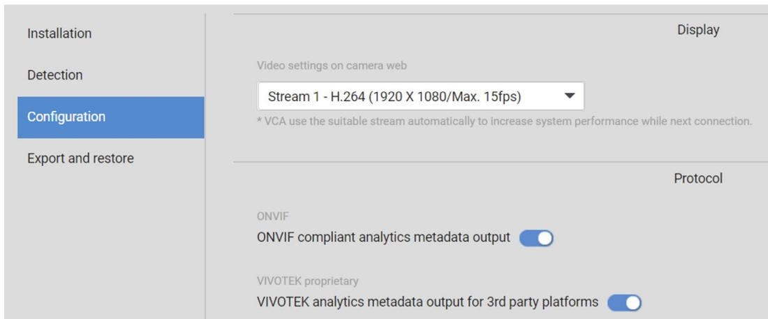
The **ONVIF** option is selected when you need to display detection details on 3rd-party software, such as Milestones. The metadata is sent to the VMS using the ONVIF protocols. Another option is for the analytics data to be ported to a 3rd-party platform, displaying detection results on video management software.
