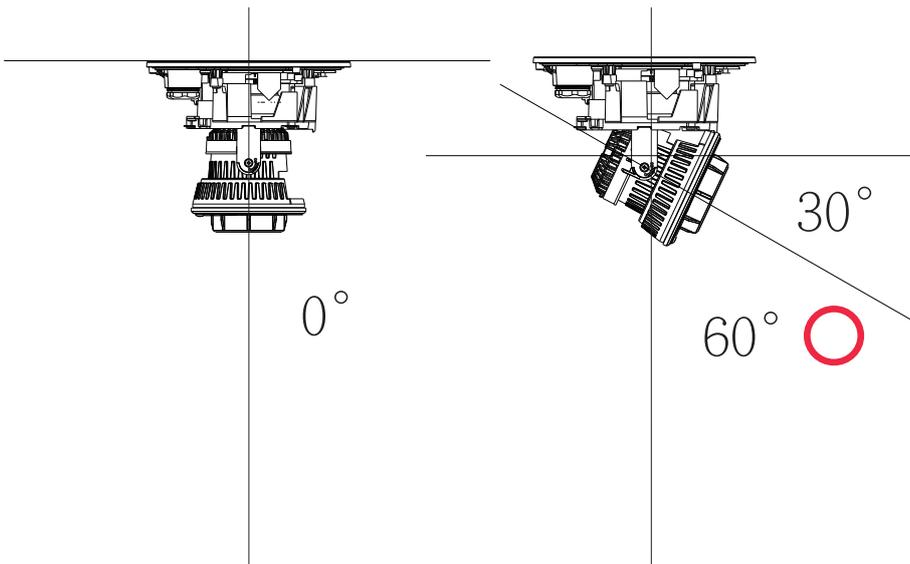
The roll angle is one that refers to the horizontal level line.
