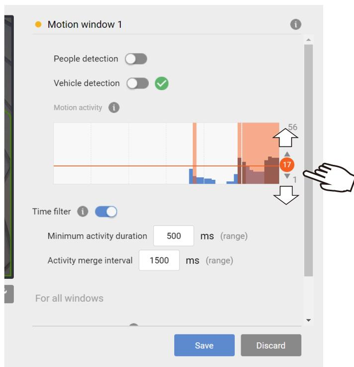
The Motion sensitivity can be associated with object sizes. The higher the sensitivity, the smaller the object size can be detected. Change the trigger level if necessary, judging from the live view of your scene.
