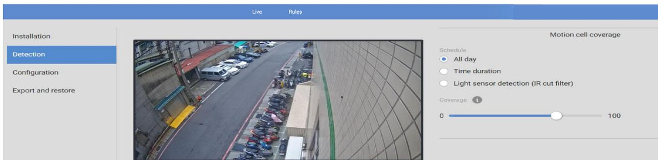
Depending on the different lighting conditions throughout a day, you can configure a different sensitivity for a specific span of time and individually for People detection, Vehicle detection, or Object detection. For day or night modes, you can configure different sensitivity settings in terms of [Less false alarms](#) or [Less missing people](#)(or Vehicle or Objects).
