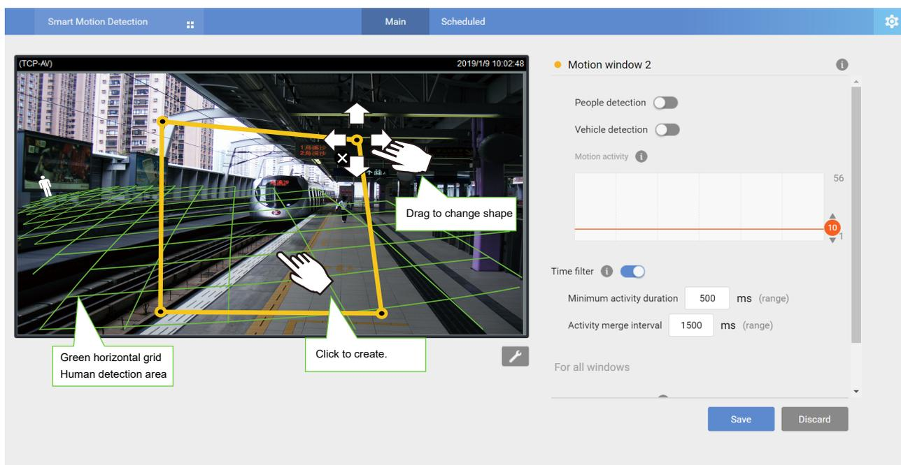
Change the coverage area of the window by dragging the corner marks. Note that the coverage area should comply with the Human detection area. The Human detection area is indicated by the red, dotted line.
