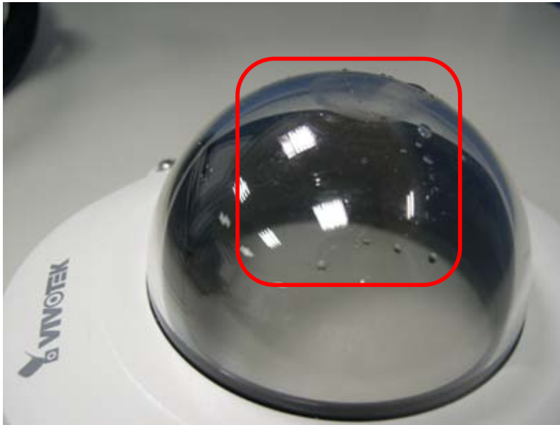
IR reflection caused by fogging of the cover
