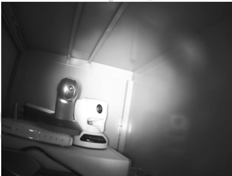
IR reflection caused by fogging of the cover
